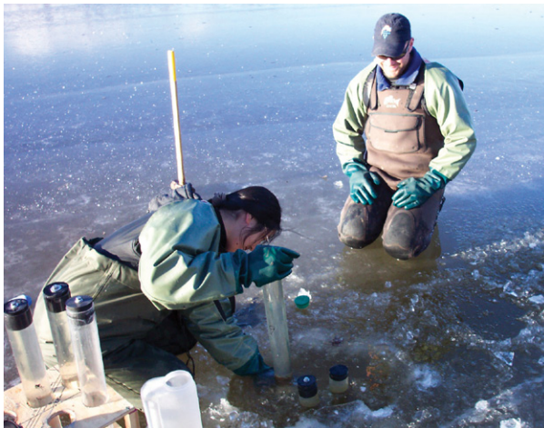
DEPOSITIONAL SEDIMENT CORES ARE COLLECTED FROM THE UPPER ATHABASCA RIVER TO BETTER UNDERSTAND THE COMPOSITION OF RIVER SEDIMENT. THIS INFORMATION HELPS THE PROVINCE MANAGE THE IMPACTS OF OIL SANDS DEVELOPMENT.
